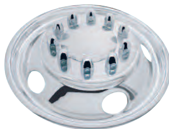
20311 24 1/2" O.D. 5 Hand/Vent Holes Stud Piloted
